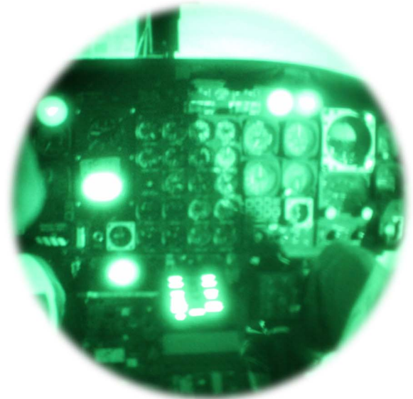
Example of what you will see through NVG-104 Inspection Scope in a non compatible cockpit.
